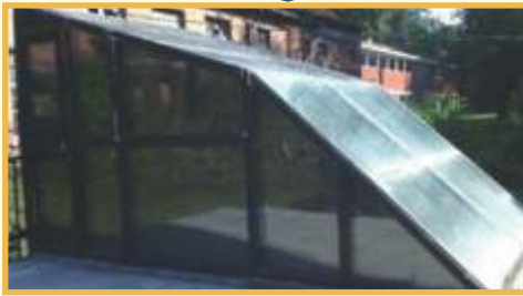
Head based storage Solar Kiln
